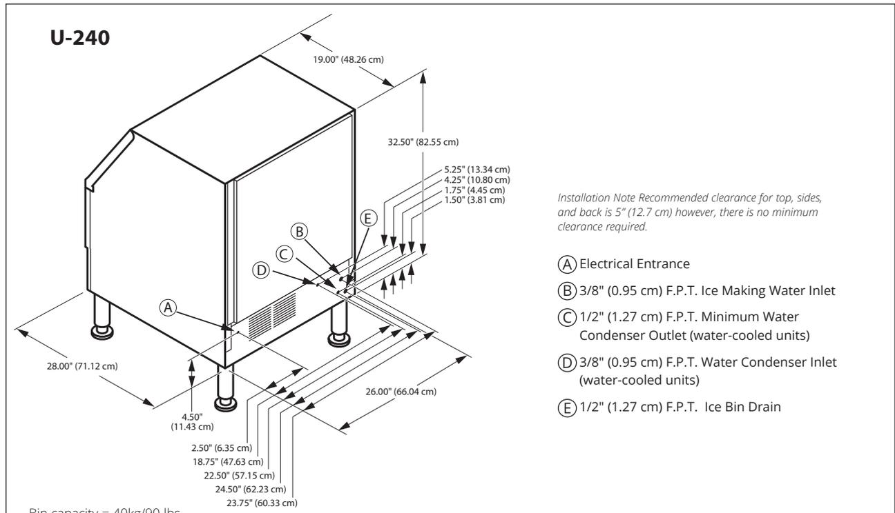
*Installation Note Recommended clearance for top, sides, and back is 5" (12.7 cm) however, there is no minimum clearance required.*
