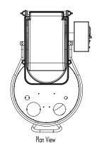
Line drawing is the SL300RB SL250RB SL300RB Α 52 7/8" (134.3cm) 52 7/8" (134.3cm) В 79 1/4" (201cm) **79 1/4"** (201cm) С 58 3/8" (148.1cm 58 3/8" (148.1cm 89 7/8" (228.1cm) 89 7/8" (228.1cm) 76 1/2" (194cm) 76 1/2" (194cm)
