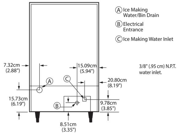
**Installation Note** - There is no minimum clearance required, however recommended clearance for top, sides, and back is 5" (12.7 cm).
