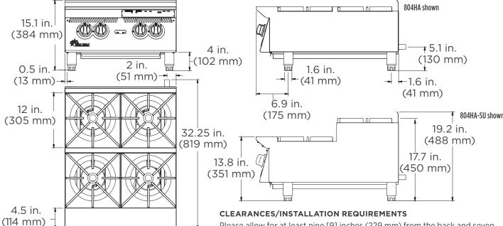
Please allow for at least nine [9] inches (229 mm) from the back and seven [7] inches (178 mm) from each side between the unit and any combustible surface.
